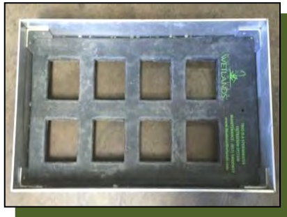
Refilling tray for media replacement.
