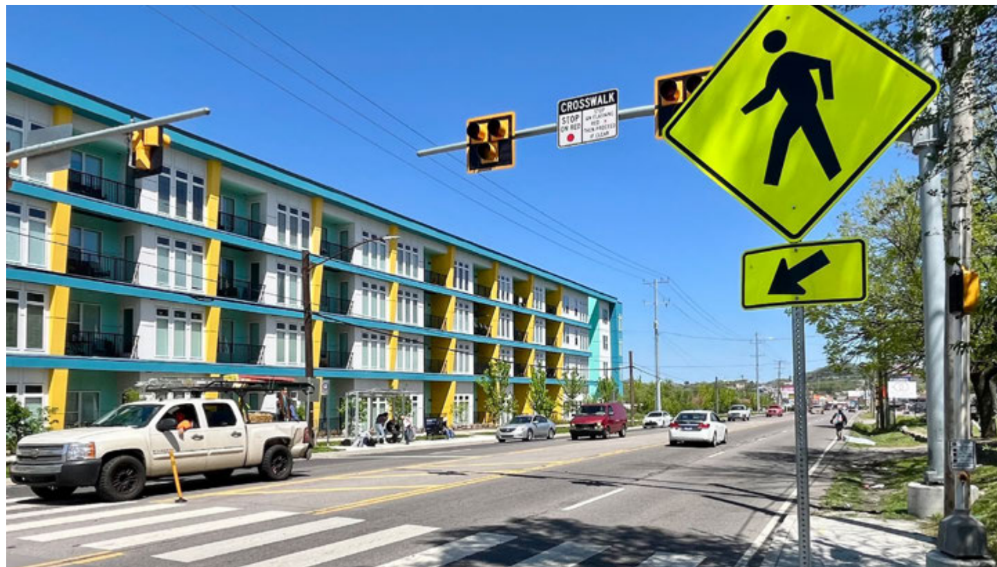
All-Access Corridors feature safety upgrades like these HAWK signals on Dickerson Pike
