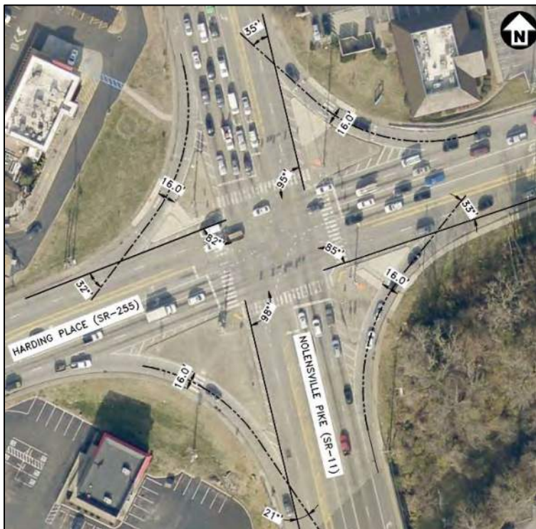
FIGURE 1 – EXISTING SLIP LANE GEOMETRY AT NOLENSVILLE PIKE (SR-11) & HARDING PLACE (SR-255)
