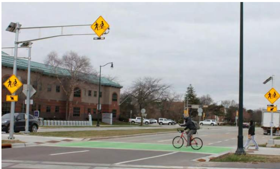
Example of Overhead & Pole Mounted RRFB Devices (Source: TAPCO)
