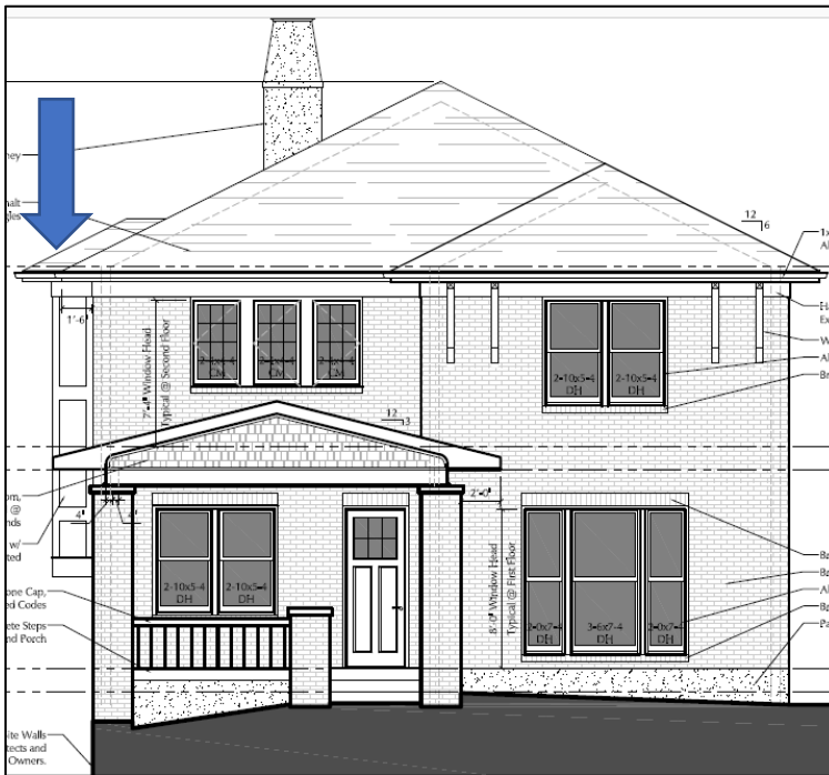
Figure 2. The front elevation showing the side bay that will encroach two feet (2') into the Beechwood Avenue side setback.
