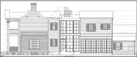
Figures 7 & 8. South elevation of main house and log house today above, and proposed with new connector, below.
