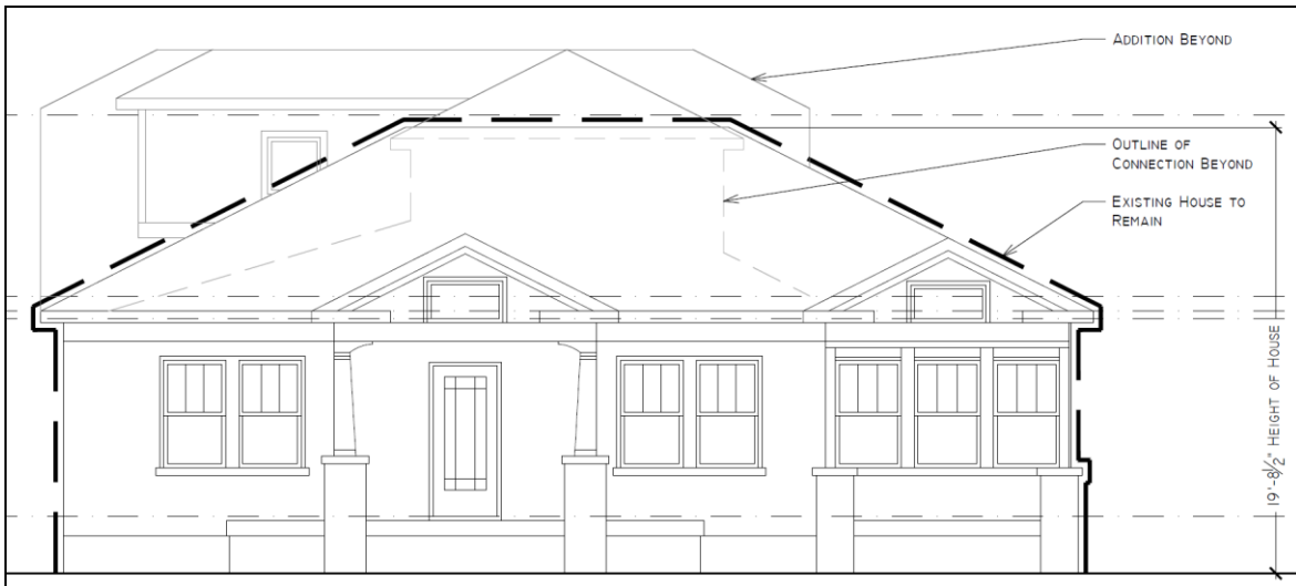
Figure 3. Proposed front elevation with addition.
