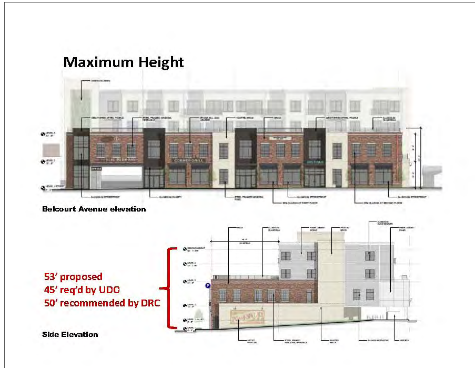
Figure 2: Elevations of building
