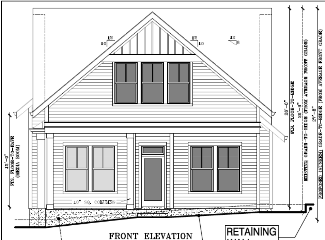
Figure 2. Proposed front elevation. The dotted line indicates existing grade, which will be dug out.
