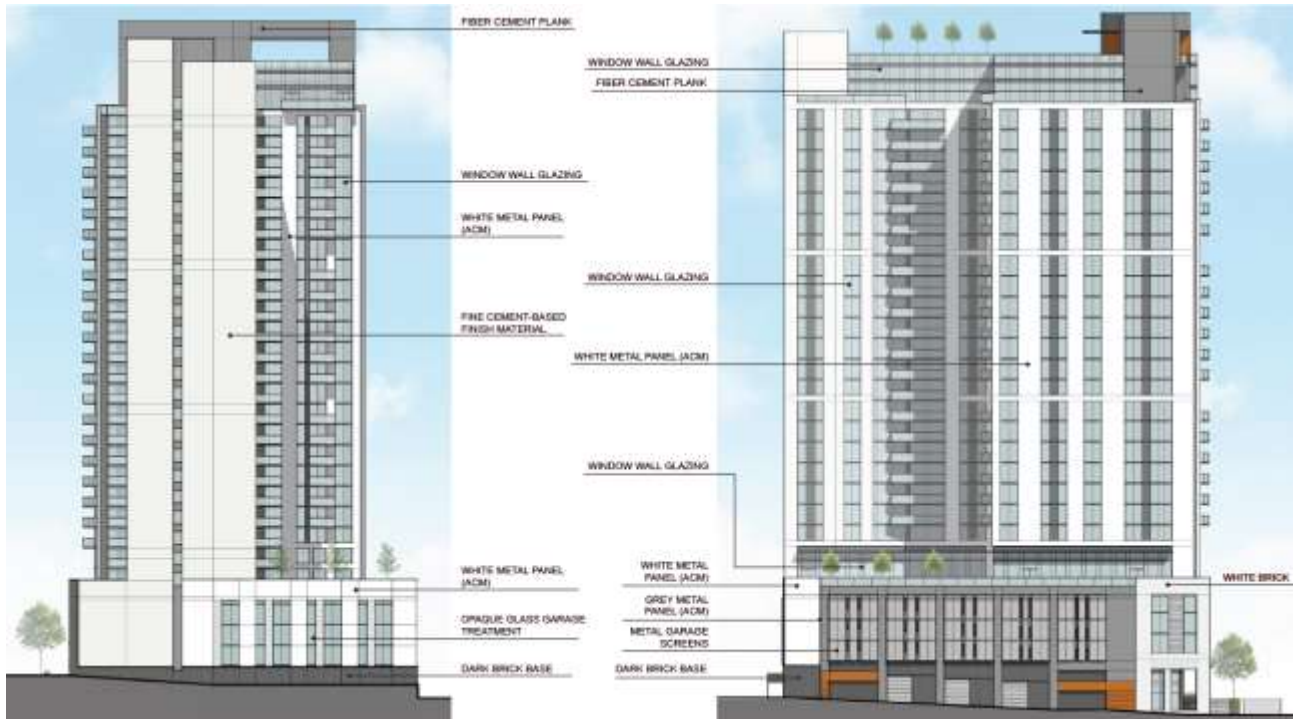
Figure 3: East Elevation (left) and North Elevation (right)
