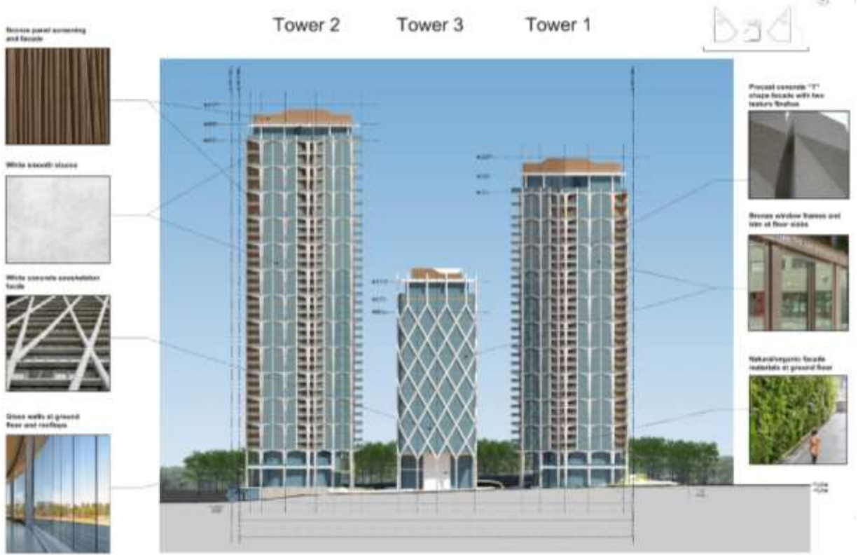
Figure 3: Elevations and Materiality
