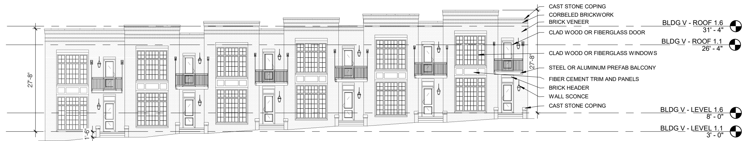
2 East Elevation - Building V 1/16" = 1'-0"
