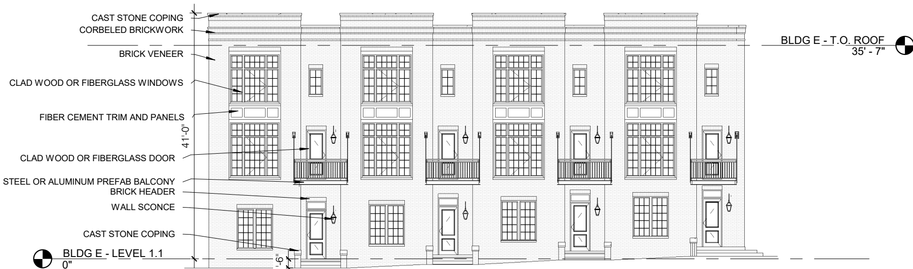
1 South Elevation -Building E 1/16" = 1'-0"
