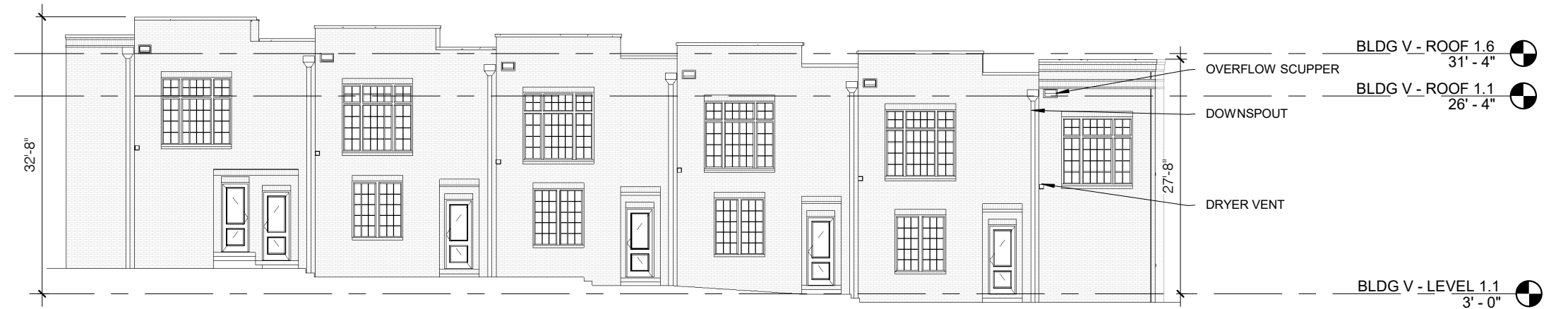
1 West Elevation - Building V 1/16" = 1'-0"
