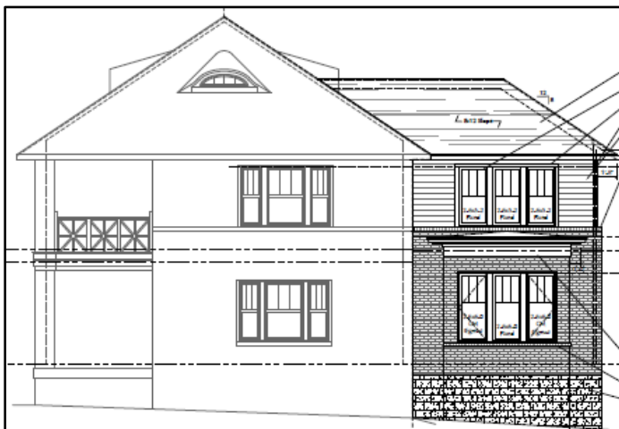
Figure 4: Front elevation showing side addition
