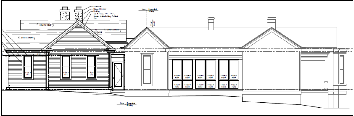
Figure 6: 9 th Street elevation. Rear addition is sixty-four feet (64') back with a separate roof form
