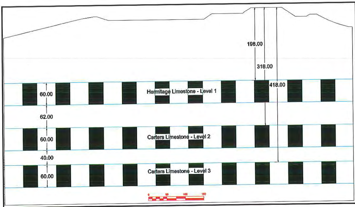
Figure 3. Cross Section of the Initial Three Levels of the Whites Creek Mine
