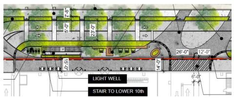
Figure 5: Vertical Circulation between Upper and Lower 10<sup>th</sup> Avenue North
