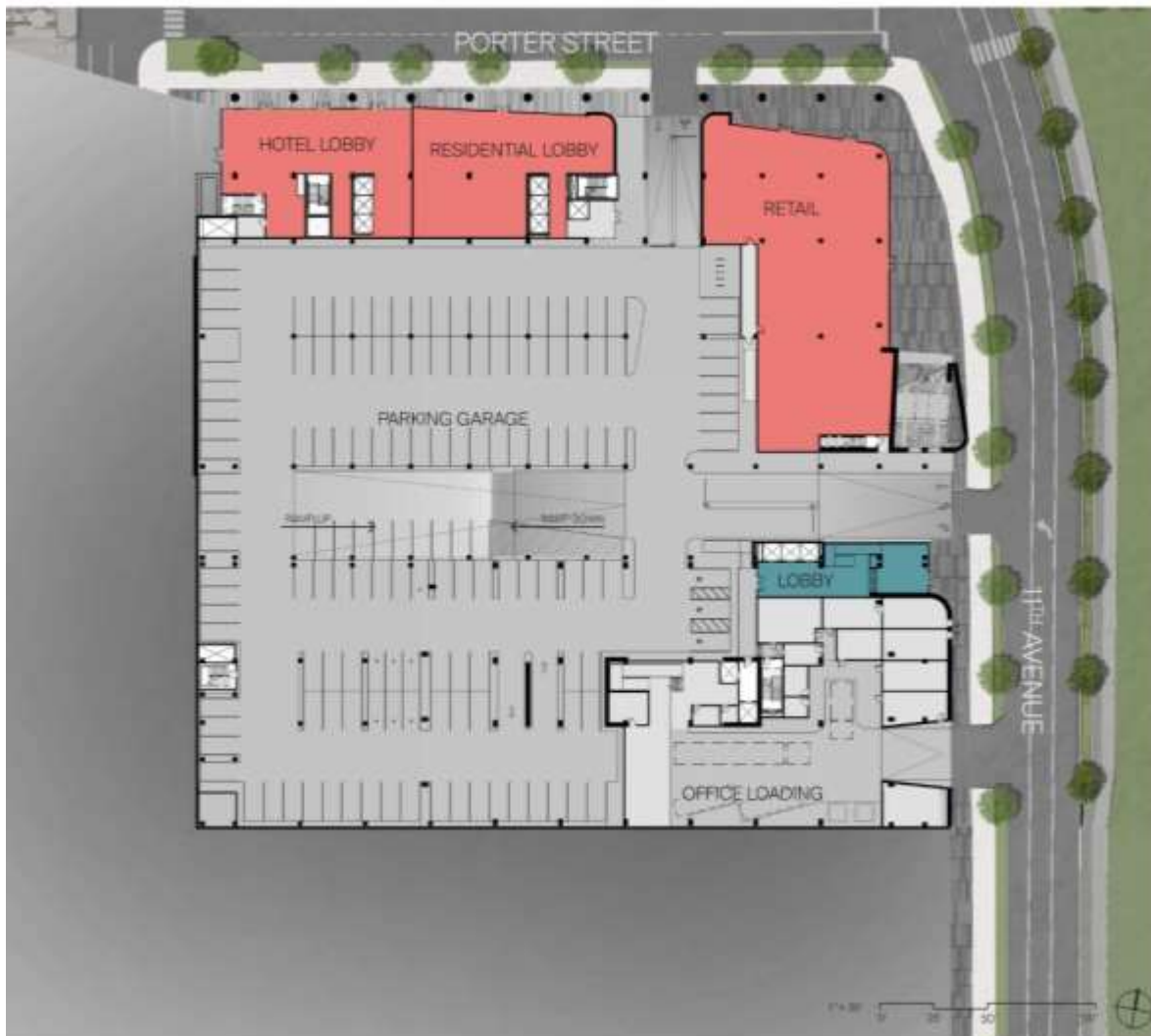
Figure 3: This lower-level site plan (11 th Ave. and Porter St.) illustrates that the garage at the lower level is lined with active uses on Porter Street and 11 th Avenue.
