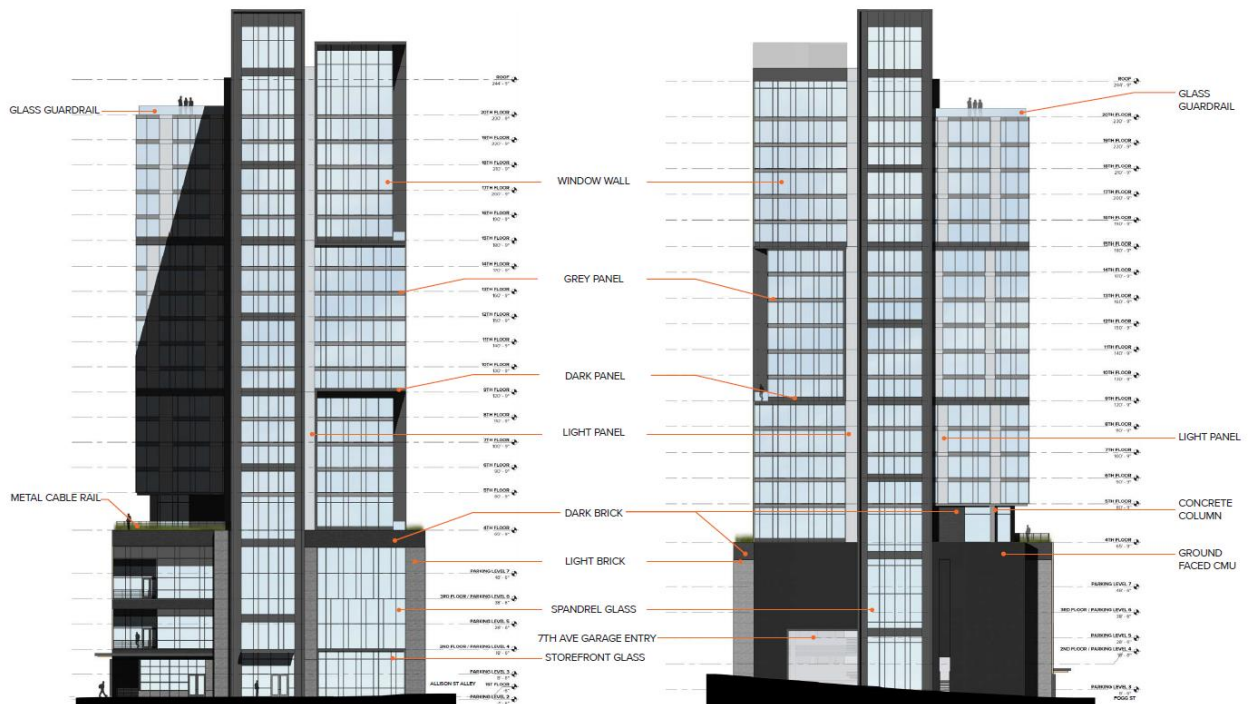
Figure 4: West Elevation (left) and 7 th Avenue South Elevation / East Elevation (right)
