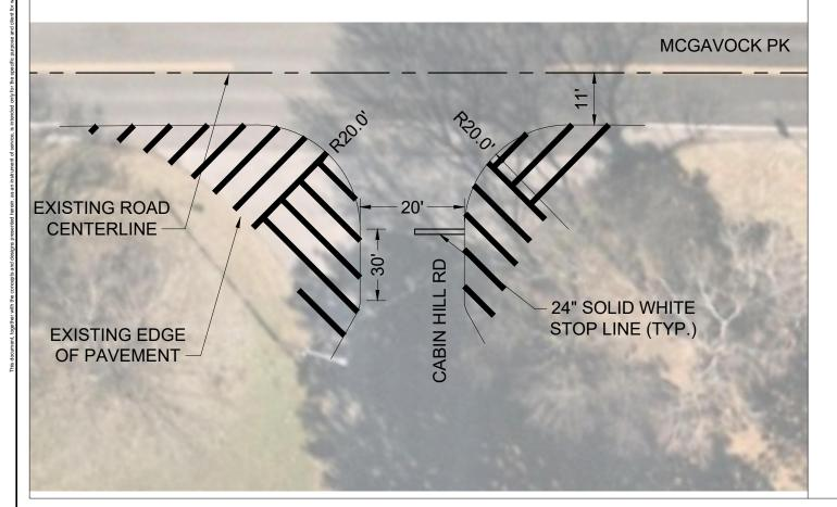
Drawing name: K-WSH\_TPTO/118900048 - Traffic Calming/3 - Design/24 - Cabin Hill Rd/Design/CAD/Plansheets/CABINHILLROAD-TrafficCalming.dwg\_06-DETAIL\_Jul 25, 2024\_10:03am\_by: Ryan.Sie
