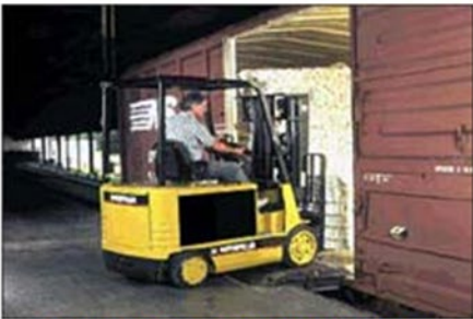
Class I: Electric Motor Rider Trucks
