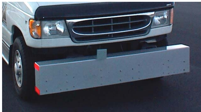
Figure 3.2. Profiler on Digital Survey Vehicle.
