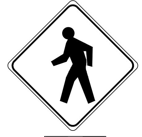
W11-2 36"x36" WITH RAPID FLASHING BEACON SIGN (S3)
