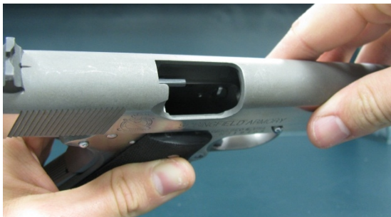
Step 3: Visually inspect the chamber
