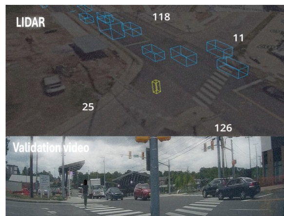
Figure 3. Top: lidar automatically detects bounding boxes of vehicles (blue) and pedestrians (yellow). Bottom: validation video used to verify count accuracy.
