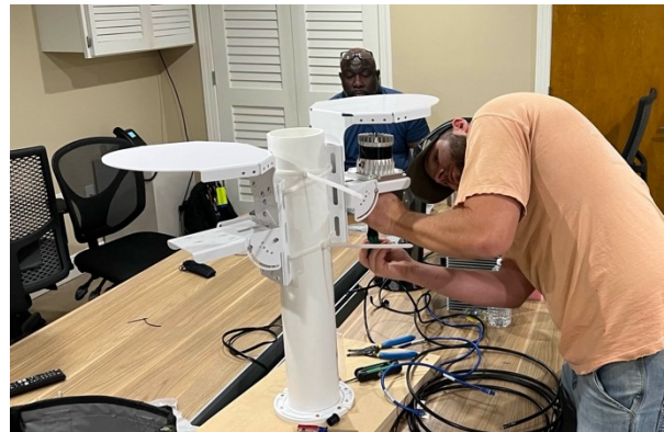
Figure 7. NABCO IBEW team member assembling a lidar unit on a test bench during a workforce training session in Chattanooga, TN.
